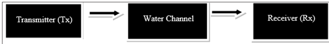
Fig 1: Block Diagram of the Wireless Underwater Communication Using Li-Fi
